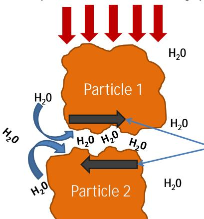
Water pressure forces water between Particle 1 and Particle 2
