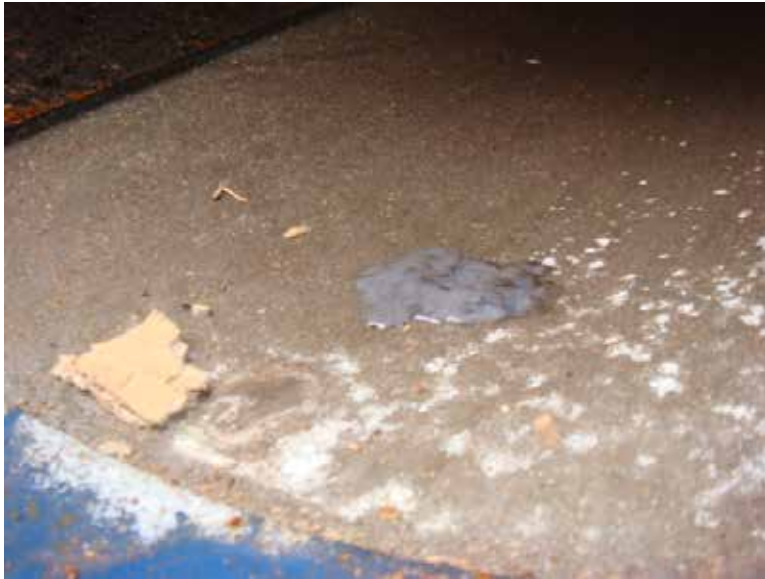
Silver nitrate testing– cargo hold
