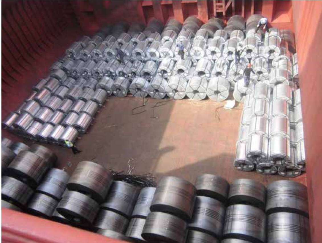
Packaged cold rolled steel coil that is well stowed.
