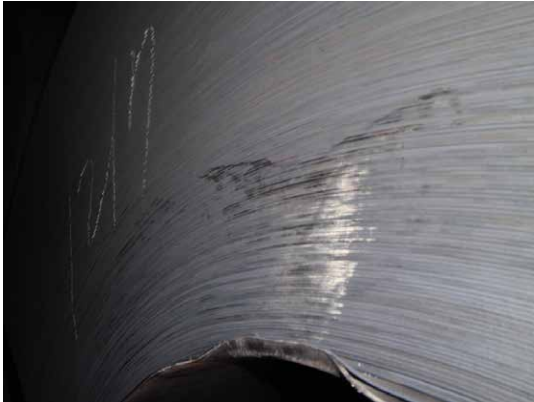
Hot rolled steel coil damaged by forklift
