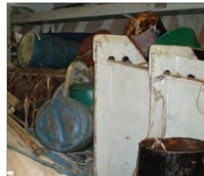
Figure 2: Timber dunnage stored in an untidy and dirty forecastle store — not how it should be stored.
