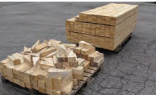
Figure 6: Timber dunnage which has been heat treated and stamped.
