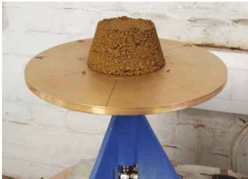
Flow table test sample for FMP and TML analysis
