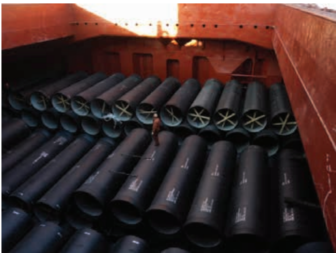
Figure 3.3 | Large diameter steel pipe with swaged ends stowed in a fore and aft direction. Note the pipes are stowed such that each tier is laid in the opposite direction to ensure the swaged ends are not loaded on top of each other.
