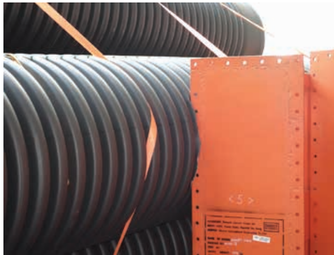
Figure 1.12 | Pipe cut due to contact with steel project cargo.
