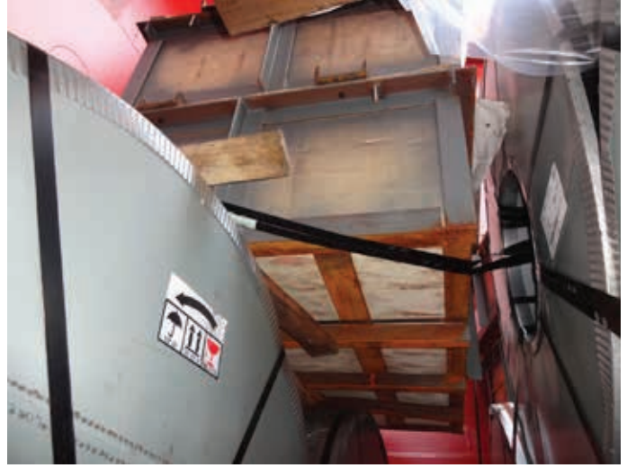
Figure 5.6 | Note that the wooden case is resting on the steel lashing bands for the steel coils.
