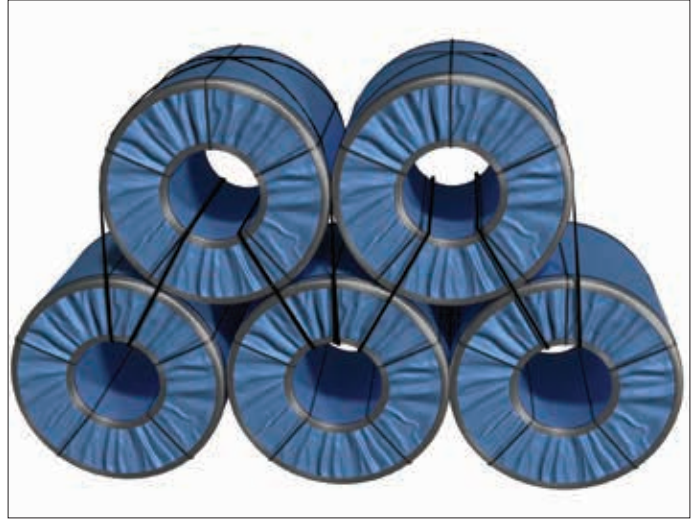
Figure 5.29 | Securing/lashing through centers of coils with 1 inch (2.5cm) wide flat steel band. Note that top-tier coils are banded in groups of threes to lower or adjacent coils depending upon the stowage configuration.
