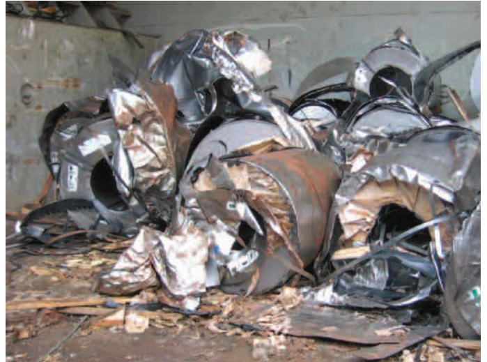
Figure 1.10 | Damage to coils due to cargo shifting.
