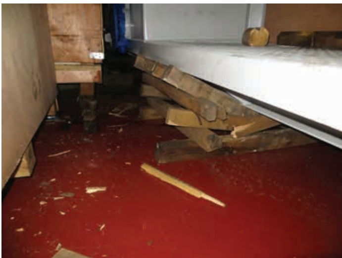
Figure 4.7 | Crushed dunnage caused the cargo stow failure.
