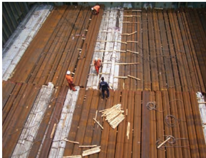
Figure 3.12 | Steel angle and steel pipes are stowed in fore and aft direction inside cargo hold.
