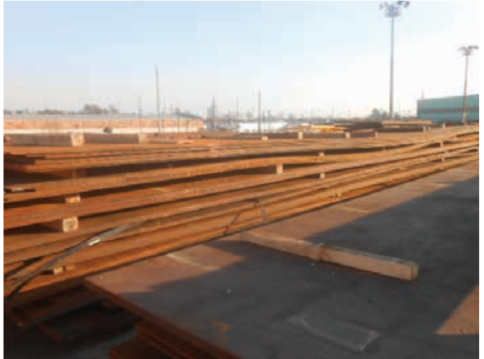
Figure 5.23 | Deformed steel plates. Note the dunnage not placed properly vertically and too far apart horizontally.
