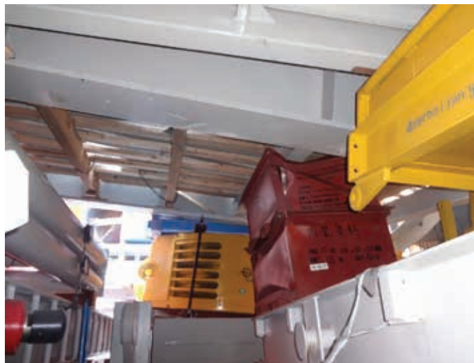
Figure 1.14 | Stowage of heavy cargo on top of steel case causing the cargo stow failure and damage to steel case cargo.
