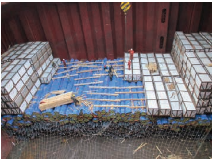
Figure 3.9 | A mixed consignment of re-bar, small diameter steel pipes and other steel products in a cargo hold.
