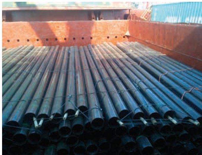
Figure 5.35 | Secured/lashed large diameter pipe. Note the dunnage wood inserted into the pipes in the foreground used for the lashing and securing of the top tier of stowed pipe.
