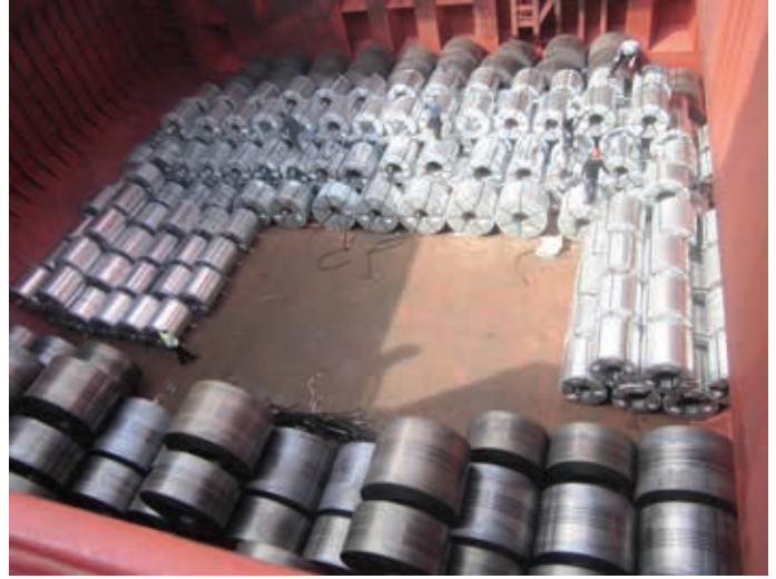
Figure 3.6 | Cold rolled steel coils being stowed and lashed with 1 inch (2.5 cm) wide flat steel bands in a cargo hold.
