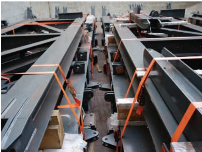
Figure 5.32 | Nylon stripping bands and ratchet tighteners used on steel “I” beams.
