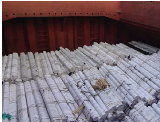
Figure 3.10 | Packaged small diameter steel pipes are stowed in fore and aft direction.
