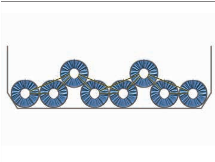
Figure 5.17 | A single-layer stowage of heavy or ultra-heavy coil with two symmetrically placed locking coils. Note additional securing/lashing of the “key” or “locking” coils in comparison for ultra-heavy coils compared to those seen in Figure 5.7 .
