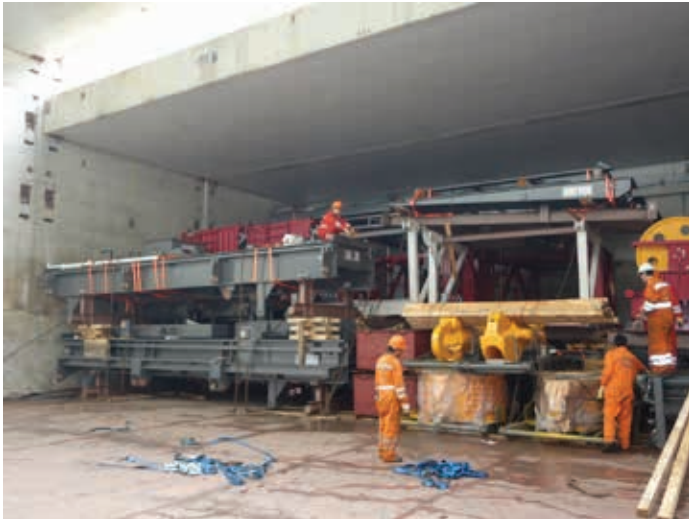
Figure 3.15 | Steel products stowed in the lower hold.
