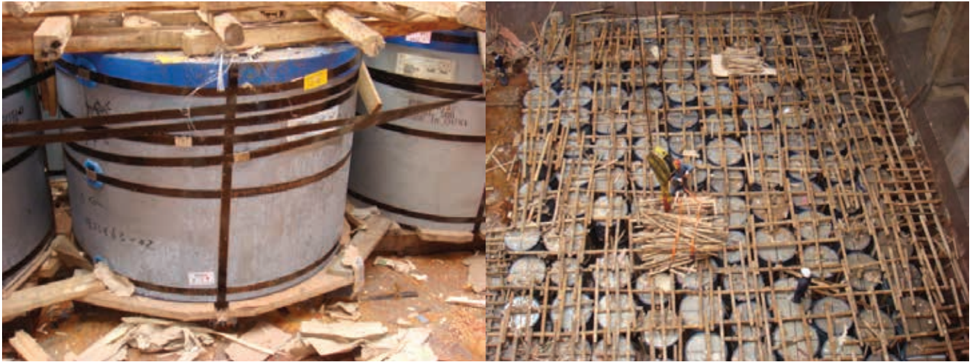
Figure 5.21 | Palletized steel coil stowed with “eye to the sky”.
