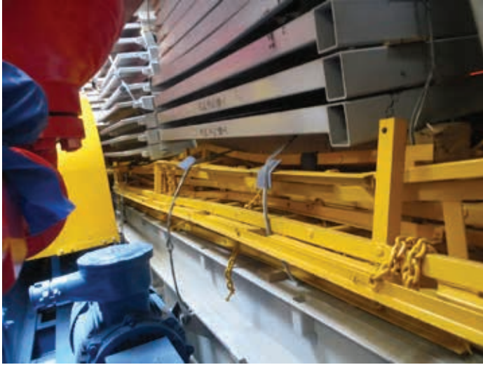
Figure 1.15 | Damage to steel products due to improper stowage and dunnage.
