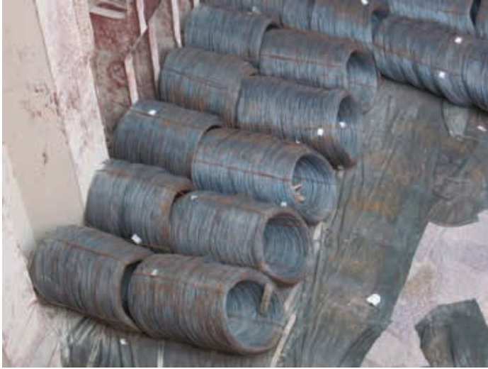
Figure 3.5 | Coiled steel wire rod being discharged. Although not a normal dunnaging practice, note the canvas tarp on tank top with wooden dunnage placed on top of the tarp.
