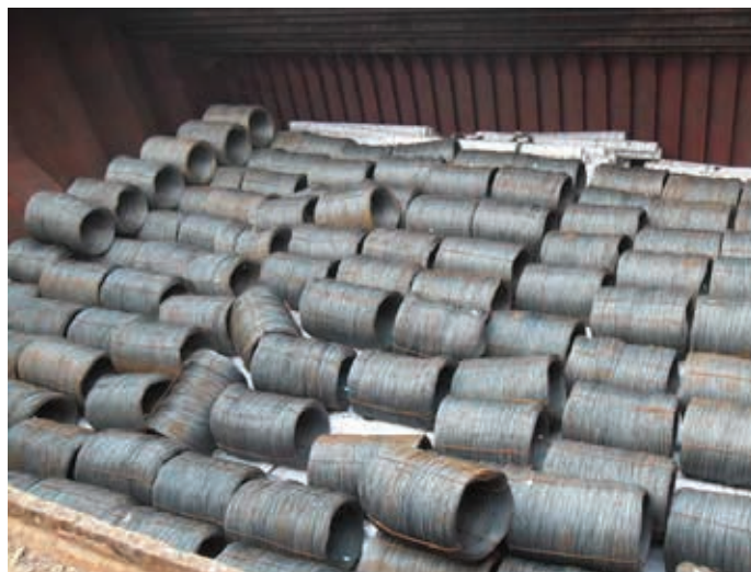
Figure 4.2 | Single and double tiers of coiled wire rod stacked on top packaged steel pipe.
