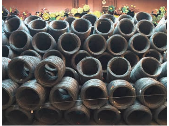
Figure 1.16 | Collapse of a cargo stow of coiled wire rods due to improper stowage and lashing.
