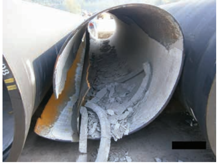
Figure 1.8 | Collapsed cast iron pipe due to crushing from other cargoes aboard the vessel.
