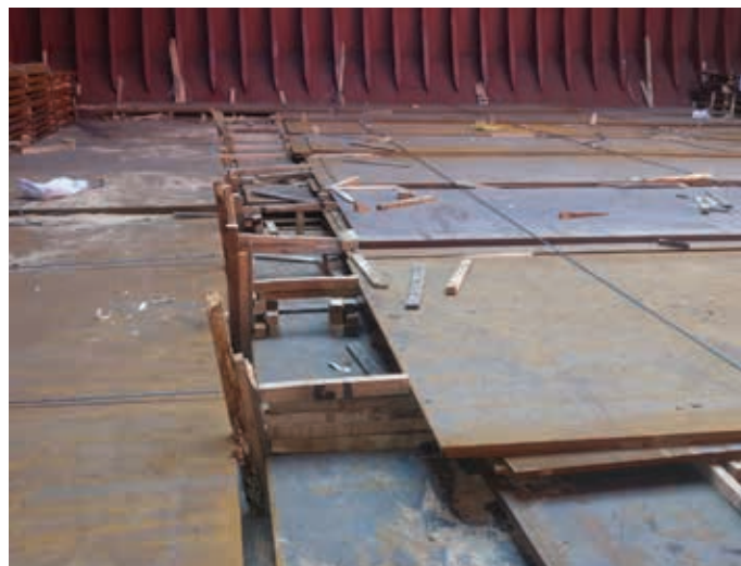
Figure 5.27 | Gaps between steel plates should be properly chocked before the vessel sails.
