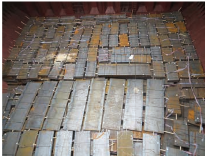
Figure 5.25 | Stowed and lashed bundled steel plate in cargo hold on tank top and hopper tanks. Note dunnage wood for long plate in foreground of picture with dunnage properly distanced horizontally to prevent deformation of plate during transit.
