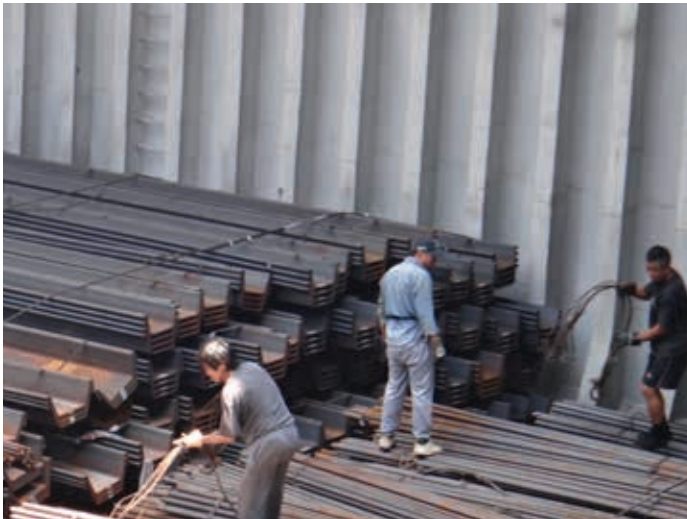
Figure 5.30 | Stevedores preparing to lash steel bar in foreground and channels. Steel channels in the background have been lashed with steel wire rope, clips and turnbuckles.
