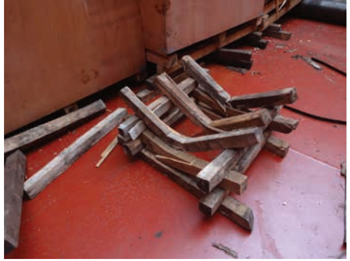
Figure 4.10 | Improper arrangement of dunnage that collapsed under the weight of the cargo.
