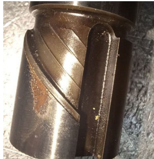
Fuel pump plunger (above) and barrel (below) with corrosion pitting marks, as a result of Singapore bunkers' usage.
