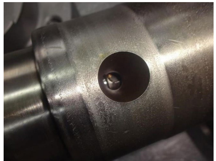
Fuel pump plunger (above) and barrel (below) with corrosion pitting marks, as a result of Singapore bunkers' usage.
