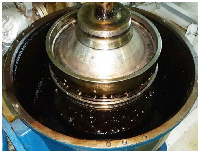
Fuel oil filter (above) and fuel oil separator (below) clogged by sludge, as a result of Singapore bunkers' usage.
