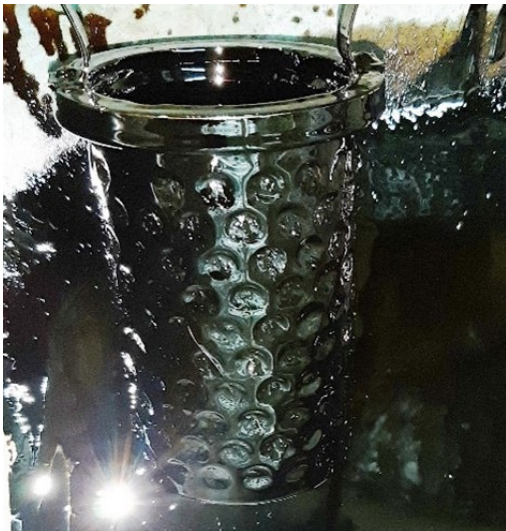
Fuel oil filter (above) and fuel oil separator (below) clogged by sludge, as a result of Singapore bunkers' usage.
