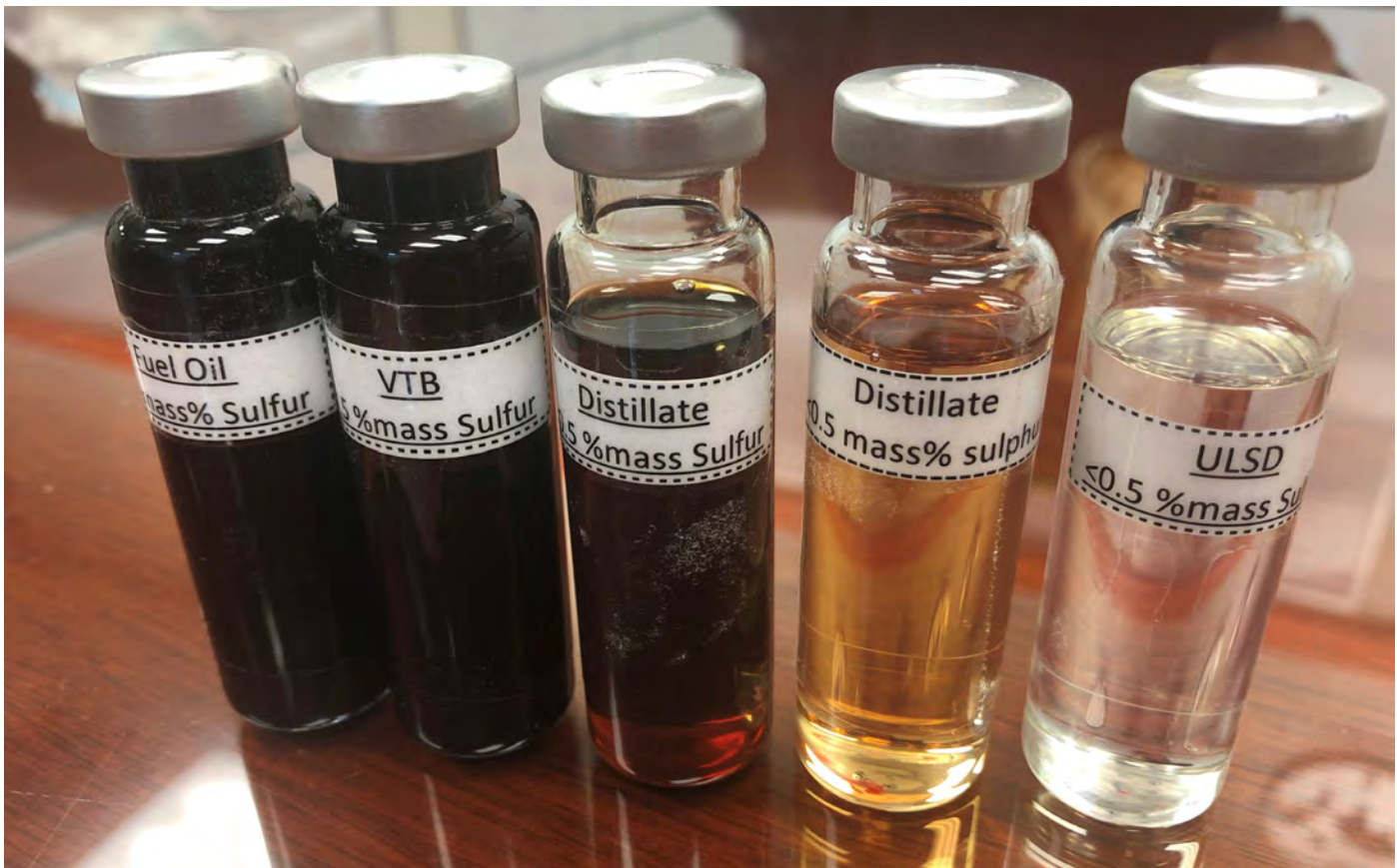
Figure 4.1 | Range of <0.5% sulfur samples including marine fuel oil, vacuum tower bottom (VTB), two distillates and ultra-low sulfur distillate.
