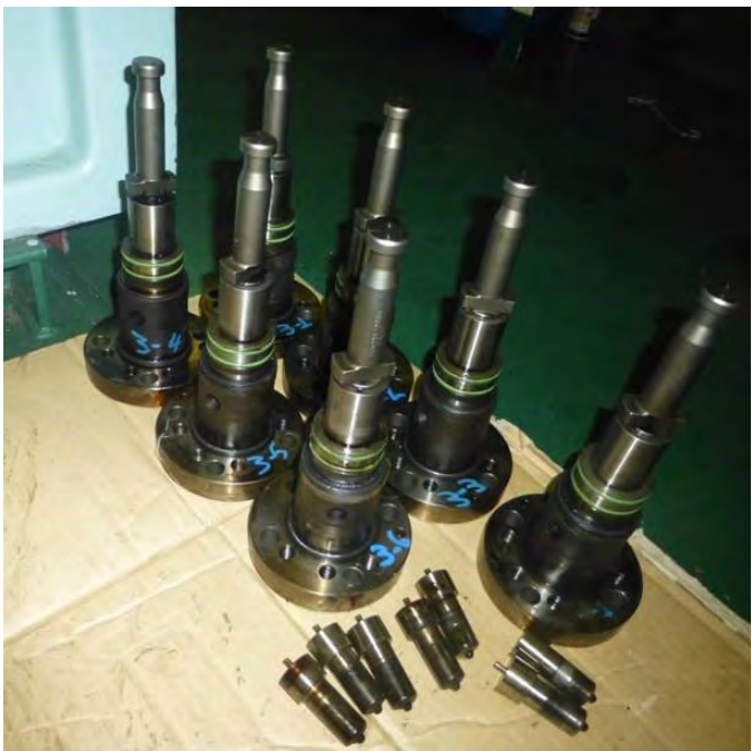
Figure 2.2 | Clean and new fuel pump plungers and injection nozzles ready for replacement of the damaged components
