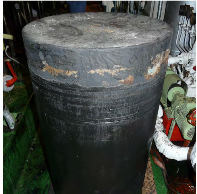
Figure 2.6 | Piston crown & rings heavily carbonized
