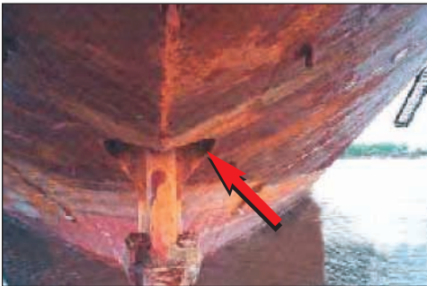
Figure 1: Stowaways climb the rudder stock into the rudder stock recess
