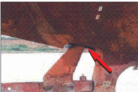
Figure 2: Rudder stock recess area where stowaways are hiding
