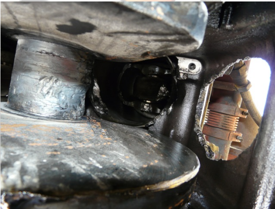
Severe crankshaft damage from breakdown of lubricating oil in a medium speed engine
