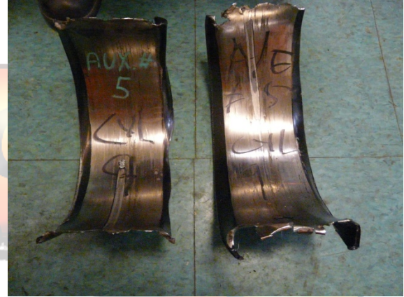
Typical bearing condition – all white metal removed
