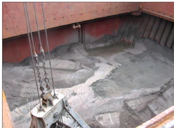
Lead concentrate in bulk, wet damaged as a result from leaky hatch covers
