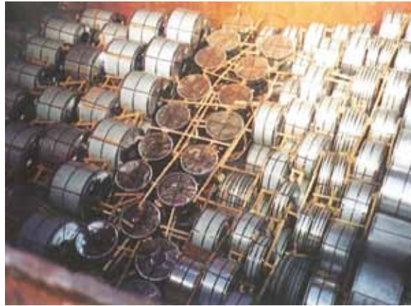
Figure 5: Steel coils stowed in the hold of a bulk carrier.
