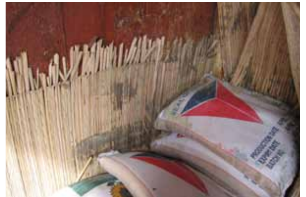
Figure 7: The ship's side plating here has been covered with matting and the bags of rice are against the matting which is against the steel plating. As a consequence the bags of rice have suffered wetting from condensation running down the cold steel.
