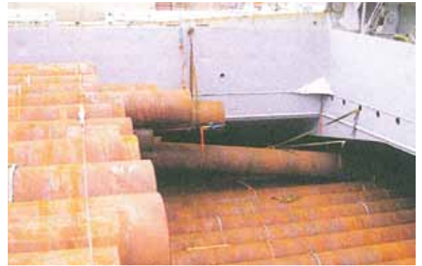
Figure 6: These upper tier pipes have suffered wetting and rusting as a result of condensation which developed because timber dunnage used lower in stowage was damp.
