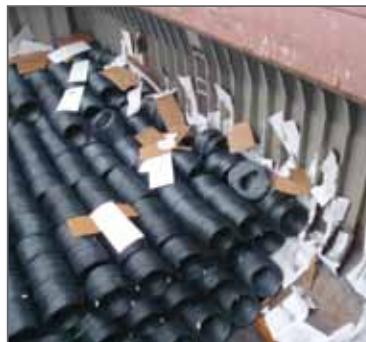
Figure 1: Stowage of steel coils in the cargo hold with cardboard dunnage provided along the bulkhead.
