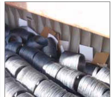
Figure 2: Steel coils compressed against cardboard dunnage on the bulkhead.
