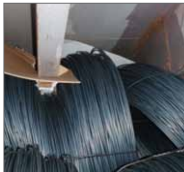
Figure 3: Steel coils damaged by compression against the bulkhead.
