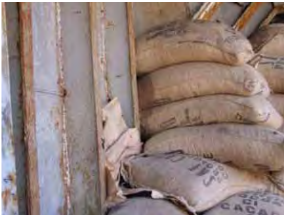
Figure 5: A further example where bags have come into contact with the shell plating and been wetted.
