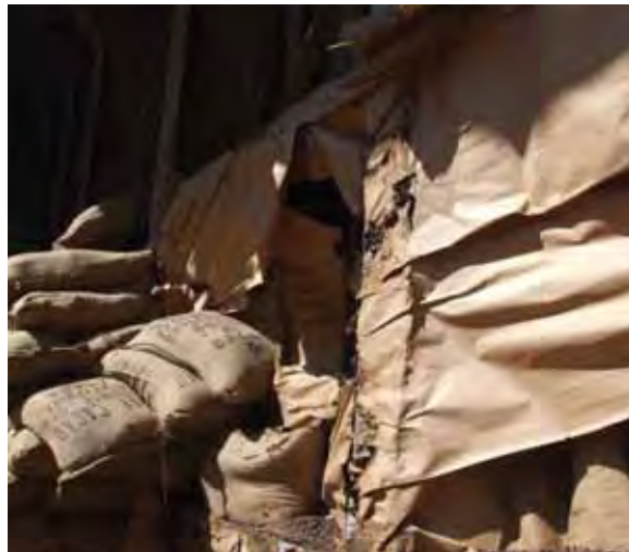
Figure 3: Kraft paper used on its own to dunnage a cargo of bagged cocoa. This was inadequate; staining and mould can be seen on the paper.
