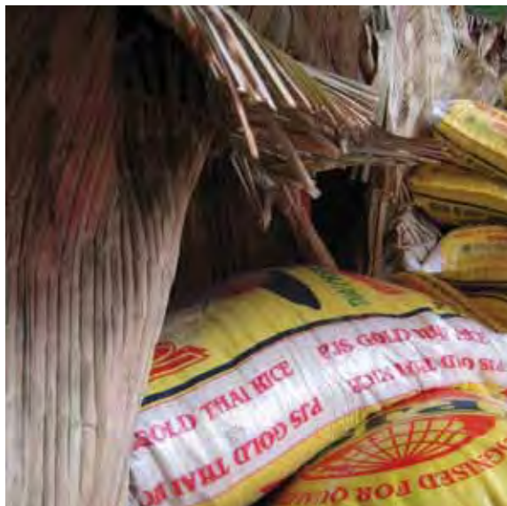
Figure 2: The same cargo as shown in (1). Bags were able to fall between the poles and, where they came into contact with the shell plating, even though there was a lining of matting the bags became wet and mouldy, as can be seen on the bag in centre view.
