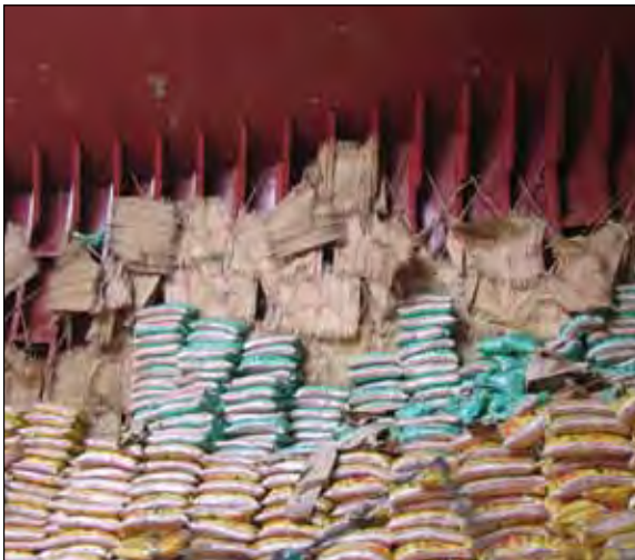
Figure 1: Bamboo poles and bamboo mats used in dunnaging a cargo of bagged rice from Thailand to West Africa. Many of the poles are flimsy, they are widely-spaced, and the dunnaging is inadequate.
