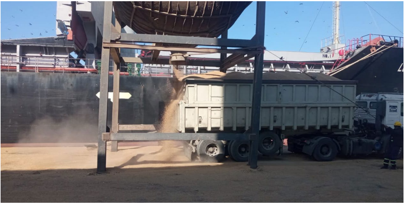
Figure 1 | Bulk grain falling off of truck and spread along quayside during discharge (c/o Budd Algiers)
