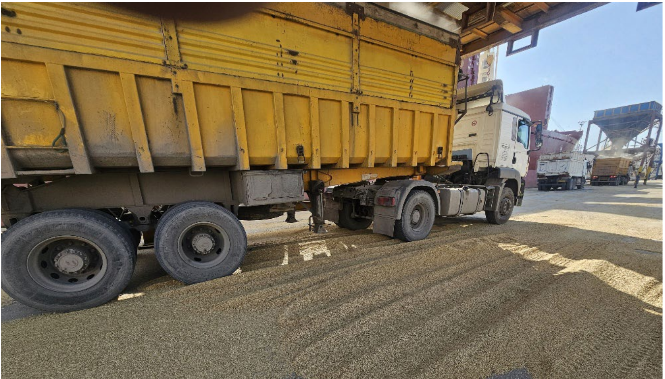
Figure 13 | Significant volumes of bulk cargo can be lost under loader transferring to trucks (c/o Budd Algiers)
