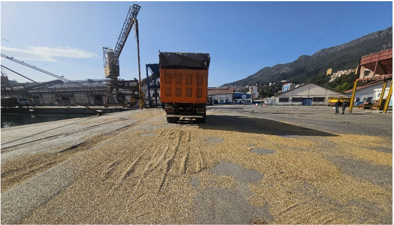
Figure 12 | Cargo falling off of trucks can lead to loss beyond the immediate quayside (c/o Budd Algiers)
