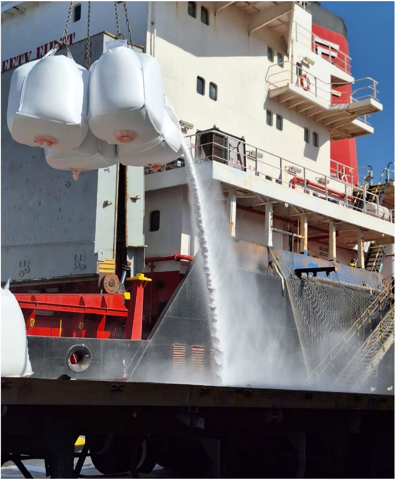
Figure 9 | Cargo spilling from torn polypropylene bags during discharge (c/o Budd Algiers)
