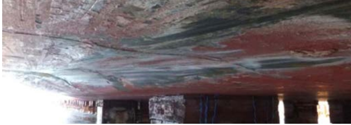
Damage to propeller and bottom of the hull due to grounding
