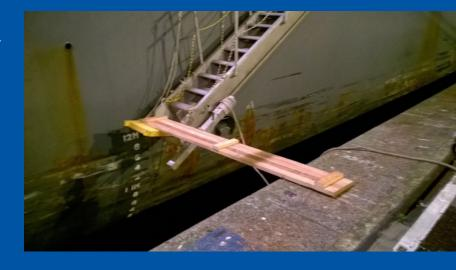
an audit of their SMS to be conducted prior to the vessel departing because they viewed this as a major nonconformity in the SMS because the embarkation arrangement was so dangerous.
