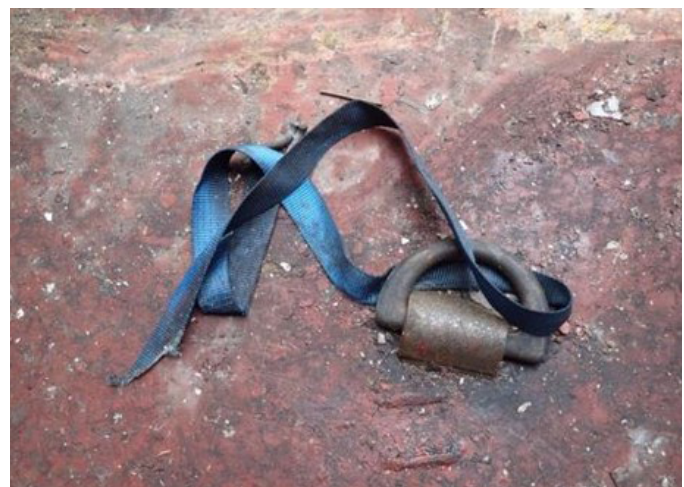
Broken cargo securing strap.
