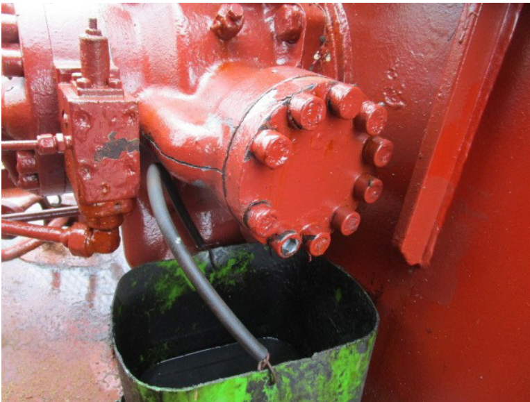
Figure 2 | Ruptured motor housing to windlass experienced during attempted recovery of anchor
