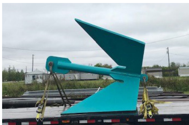
Figure 10 | Typical grapple hook used for anchor recovery
