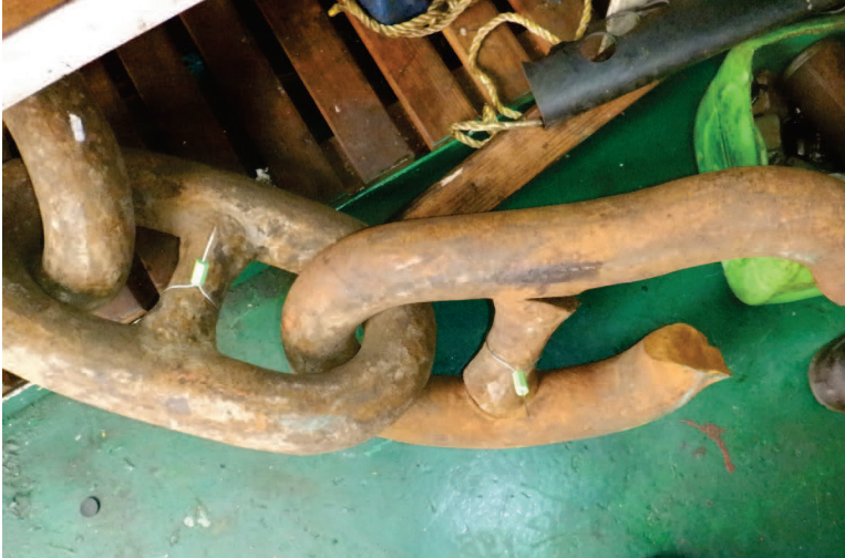
Figure 1 | Failed common link to anchor chain resulting in loss of chain and anchor
