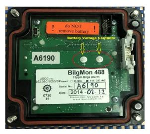
circumstances should the battery be removed. Furthermore, a red warning sticker is affixed to the circuit board as pictured above. Attempting to remove the battery in this circumstance may cause an unrecoverable error, failure and data loss. A manufacturer's representative indicated that the battery was originally designed to last the lifetime of the device and that if the RTC stops due to a power supply
