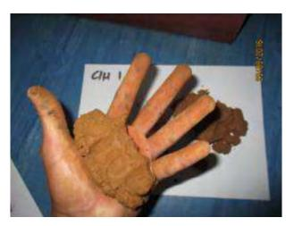
When a sample can be molded and retains a shape we say it has "Plasticised", to have the ability to do this then moisture must be present.
