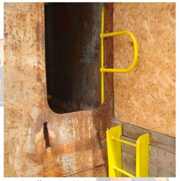
ladderwell hold design and configuration did not provide sufficient hand holds at the top of the ladder to prevent his falling. Eventually, modifications were made in order to ensure that grip bars above the ladder were installed above the ladder as seen in the figure.
