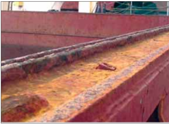
Corroded, rough and uneven compression bar
