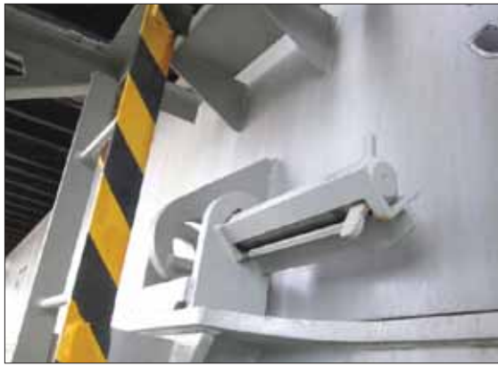
Holding down device on container vessel
